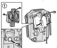
Connect the telephone line cord. Mount the unit, then slide down.
